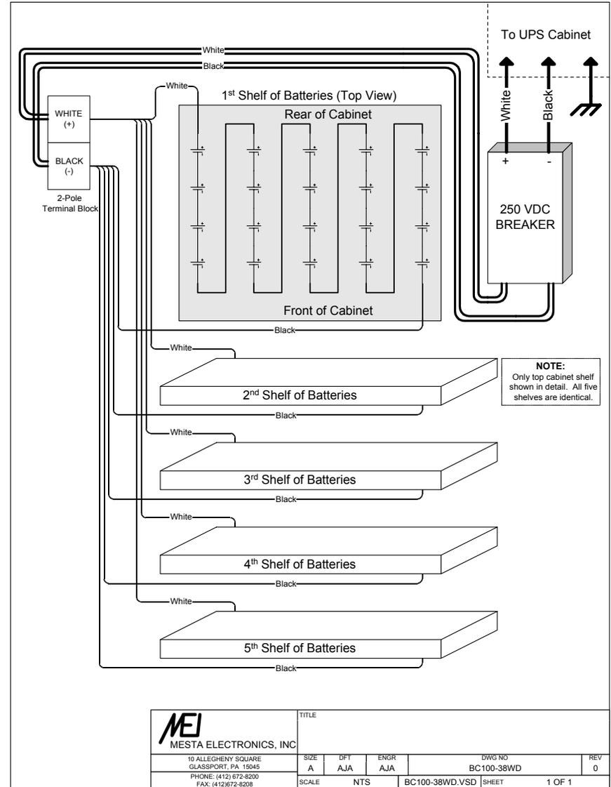
Figure 12c BC20-65 and BC40-65 Wiring Diagram
