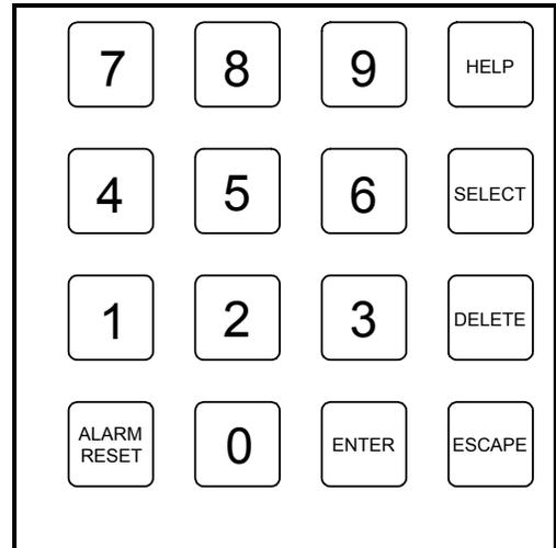
**C. DELETE key** - If a wrong number key is pressed while entering numeric data using the keypad, the DELETE key may be pressed to delete the last number entered.
