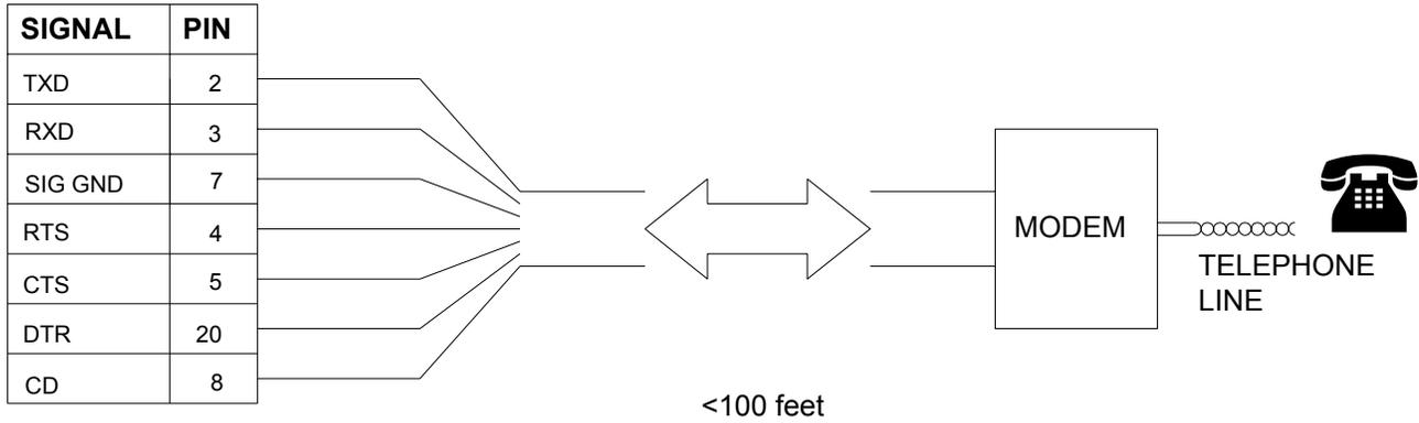
**"DTE" CONNECTOR (female - as seen on back panel):**
