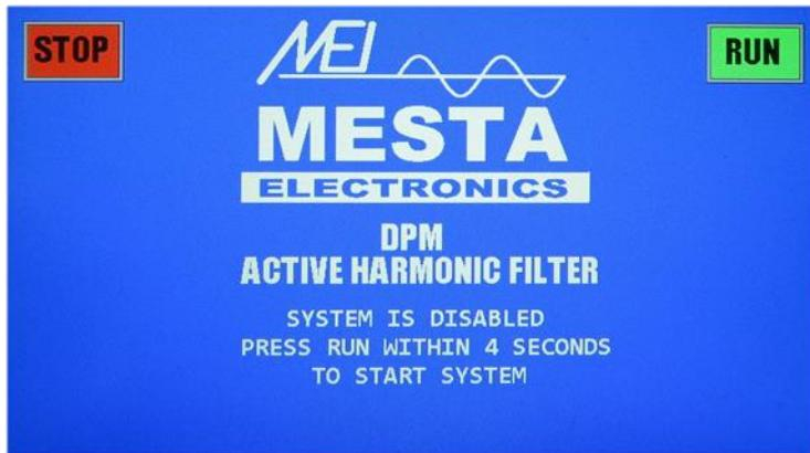
If you get the full display, you may either wait 5 seconds until the display changes to the “OPERATING STATUS” display or press the “STOP” button on the display to go to the “OPERATING STATUS” display immediately. DO NOT press the “RUN” button on the display at this time. If the display does not show anything, check to make sure 3-phase going to the DPM, or if is different than what is indicated above, contact the factory.
