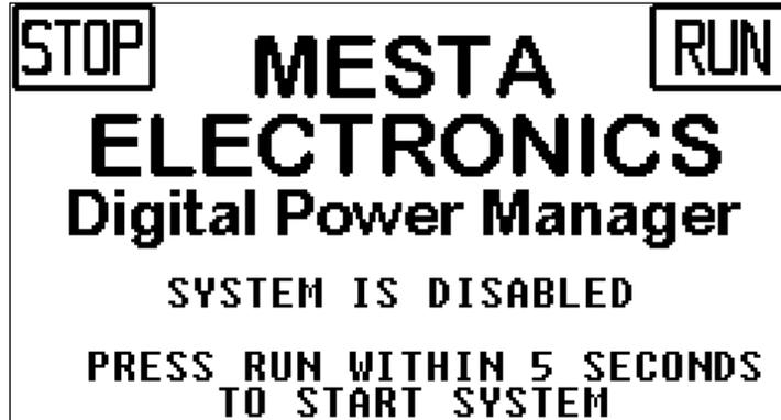
If you get the full display, you may either wait 5 seconds until the display changes to the “CURRENTS” display or press the “STOP” button on the display to go to the “CURRENTS” display immediately. DO NOT press the “RUN” button on the display at this time. If the display does not show anything, check to make sure 3-phase going to the DPM, or if is different than what is indicated above, contact the factory.
